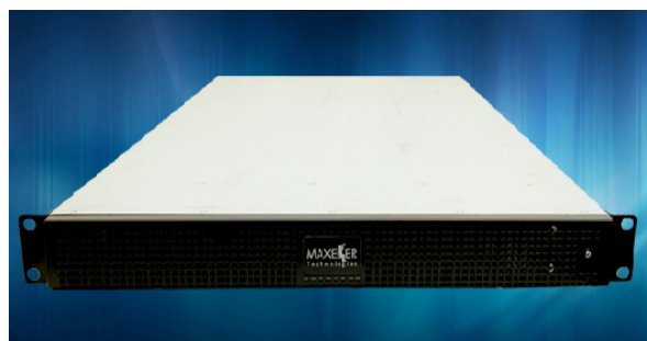
Figure 1: The MPC-X Node which serves as a building block for the Maxeler MaxRacks.
