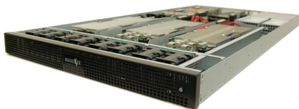
Figure 1: 1U rackable MPC-X node with 8 Dataflow Engines (DFEs) and Infiniband interconnect for communicating with standard CPU nodes running Linux via network switches.
